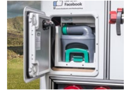
SOG toilet ventilation system
